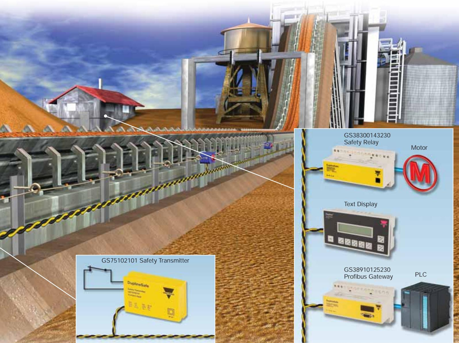
the diagnostics, but it is a difficult and costly solution, since a 3-5 km conveyor may have more than 50 switches installed. With DuplineSafe, however, a simple, flexible and cost-effective solution can be implemented.
