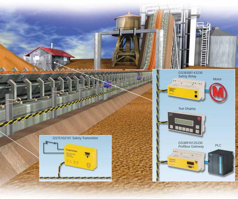
the diagnostics, but it is a difficult and costly solution, since a 3-5 km conveyor may have more than 50 switches installed. With DuplineSafe, however, a simple, flexible and cost-effective solution can be implemented.
