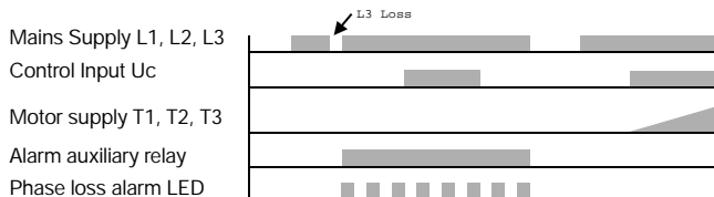
Diagram 2c: Phase loss during power up
