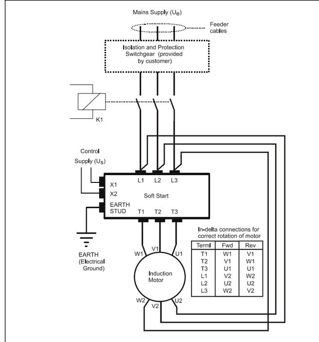
Note 2: The In-Delta configuration requires that the firing mode be set to '1'. An in-line contactor controlled by the RSXK MUST be used in the In-Delta firing mode.
