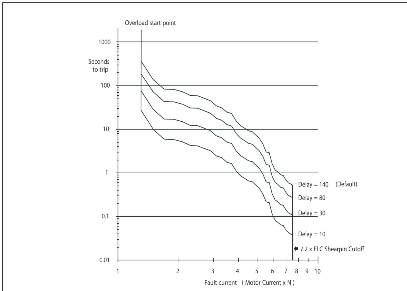
Current Limit', 'Overload level' and 'Overload delay' settings may be adjusted to limit overload currents in accordance with the trip curves shown here. For motors with FLC's lower than the rated current of the RSQK, the 'Overload Level' may be adjusted using the following formula: Overload level = Motor FLC x 1.1 (A)
