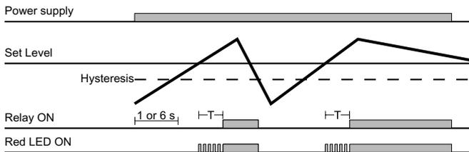
Under current - Latch function - N.D. relay
