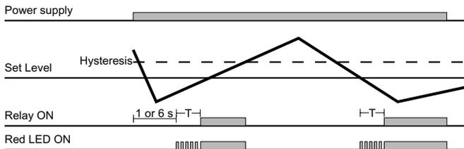
Over current - Inhibit function - N.D. relay
