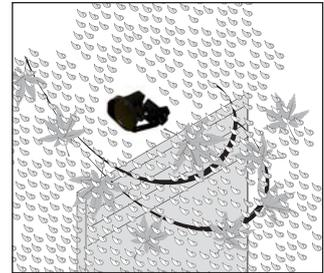
The housing of the sensor shall be concealed within a NEMA-4 type-rated enclosures and is extremely reliable in harsh environments.
