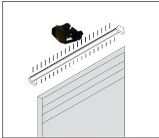
Do not install the radar close to fluorescent lamps.
