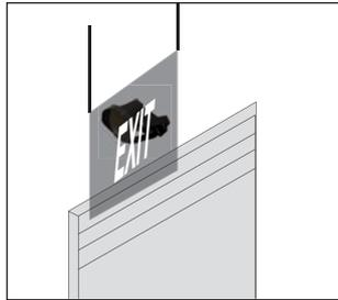
Sensor should not be placed near metal halide lights or placed behind any kind of protection layer or plate.
