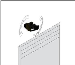
The sensor shall be firmly fixed to avoid any false activation by shocks or vibrations. It should not be mounted to high vibration surfaces such as a door canopy that houses the operating mechanism.
