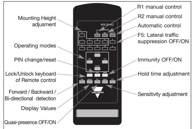
**Note:** For optimum results point the remote control at the sensor before pressing its buttons.
